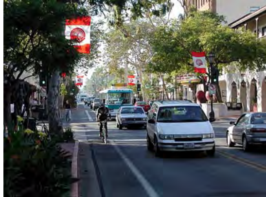
A striped bicycle lane provides a safe travel lane for bicyclists. Source: (12).
