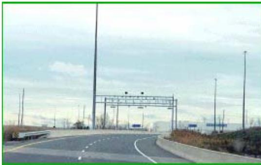
**On Toronto's Highway 407, electronic sensors located on overhead gantries log highway entry and exit points.**
