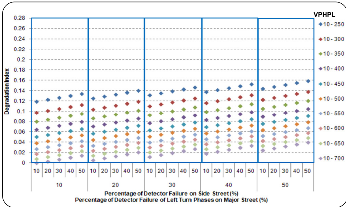
Figure 2 Degradation Index vs. Detection Failure by Different Volumes for 10% Clock Drifting
